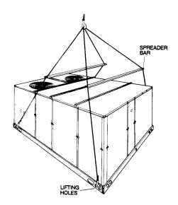
FIGURE 1 - TYPICAL RIGGING
